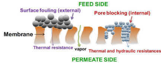
Figure 3: Surface (external) and pore-blocking (internal) fouling [8].
