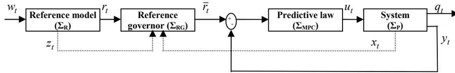
Figure 4.1: Reference governor scheme for MPC feasibility.
