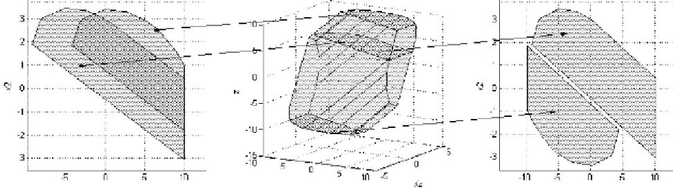
**Figure 3.2:** Example of feasible set  $\tilde{X}_f$  (center).  $\mathbf{D} = \mathbf{X}_f(\mathbf{z}_{t+1}) \cap \mathbf{X}_f(\hat{\mathbf{z}}_{t+1}) \neq \emptyset$  (left).  $\mathbf{D} = \mathbf{X}_f(\mathbf{z}_{t+1}) \cap \mathbf{X}_f(\hat{\mathbf{z}}_{t+1}) = \emptyset$  (right).
