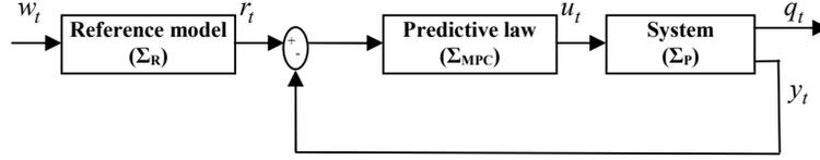
**Figure 3.1:** Classical MPC tracking scheme ( $q_t$ -the tracking quality).
