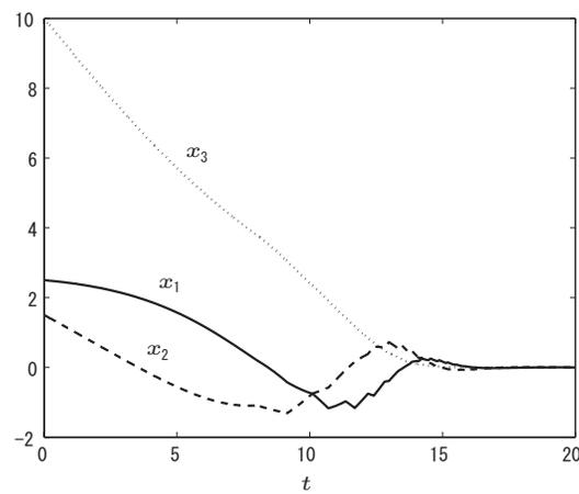
**Figure 4.3:** The states in the saturated case ( $x_1(0) = 2.5$ ,  $x_2(0) = 1.5$ ,  $x_3(0) = 10$ ).
