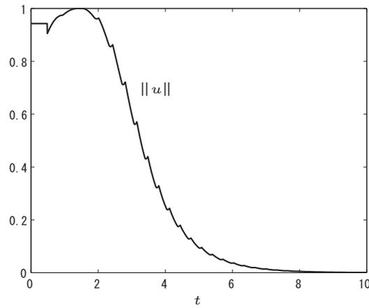
**Figure 4.2:** The norm of the control input in the saturated case ( $x_1(0) = 0.25$ ,  $x_2(0) = 0.15$ ,  $x_3(0) = 1.0$ ).
