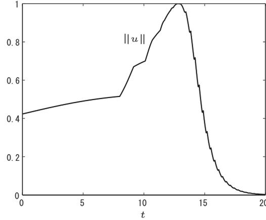
**Figure 4.4:** The norm of the control input in the saturated case ( $x_1(0) = 2.5$ ,  $x_2(0) = 1.5$ ,  $x_3(0) = 10$ ).
