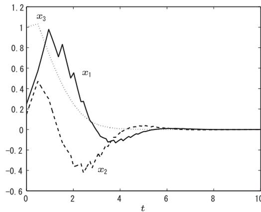
**Figure 4.1:** The states in the saturated case ( $x_1(0) = 0.25$ ,  $x_2(0) = 0.15$ ,  $x_3(0) = 1.0$ ).
