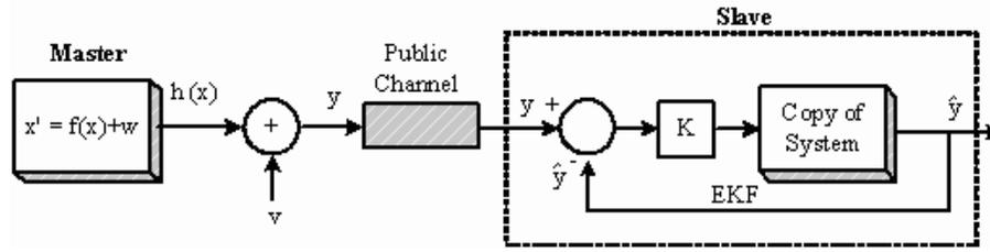
**Figure 2.1:** Master-slave coupling scheme for noisy hyperchaotic maps: where  $x' = x(k+1)$  is the state master,  $w$  and  $v$  are independent noise processes,  $y$  the coupling signal, and  $\hat{y}$  the output of EKF.
