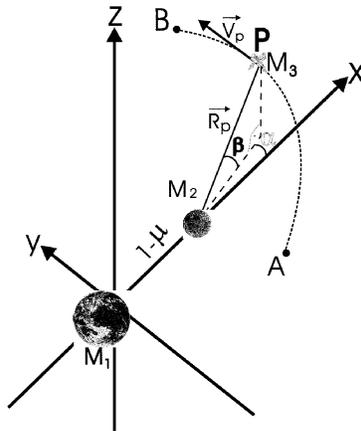
**Figure 2.1.** The swing-by in the three-dimensional space.
