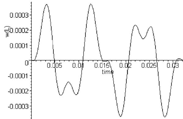
**Figure 4.2a.** Transverse displacement of free end of **delaminated** cantilever beam, excited by piezoelectric actuator. Beam length is  $L = 0.2m$ ,  $x$ -coordinates of the crack tips are  $\alpha = 0.1m$  and  $\beta = 0.15m$ ,  $z$ -coordinate of the crack tips is  $\gamma = 0.00165m$ . **Linear analysis.**
