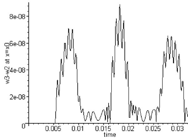
**Figure 4.3b.** Difference of transverse displacement of the upper and lower delaminated parts, at the middle of the crack's length, versus time, if the anti-overlapping constraint and the longitudinal force resultants are taken into account. **Linear analysis.**
