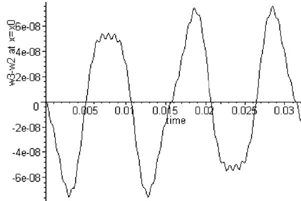
**Figure 4.3a.** Difference of transverse displacement of the upper and lower delaminated parts, at the middle of the crack's length, versus time, if the anti-overlapping constraint and the longitudinal force resultants are not taken into account. **Linear analysis.**
