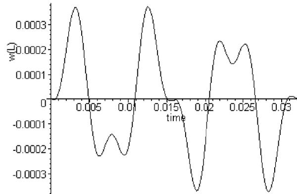
**Figure 5.1a.** Transverse displacement of free end of **delaminated** cantilever beam, excited by piezoelectric actuator. Beam length is  $L = 0.2m$ ,  $x$ -coordinates of the crack tips are  $\alpha = 0.1m$  and  $\beta = 0.15m$ ,  $z$ -coordinate of the crack tips is  $\gamma = 0.00165m$ . **Linear analysis.**
