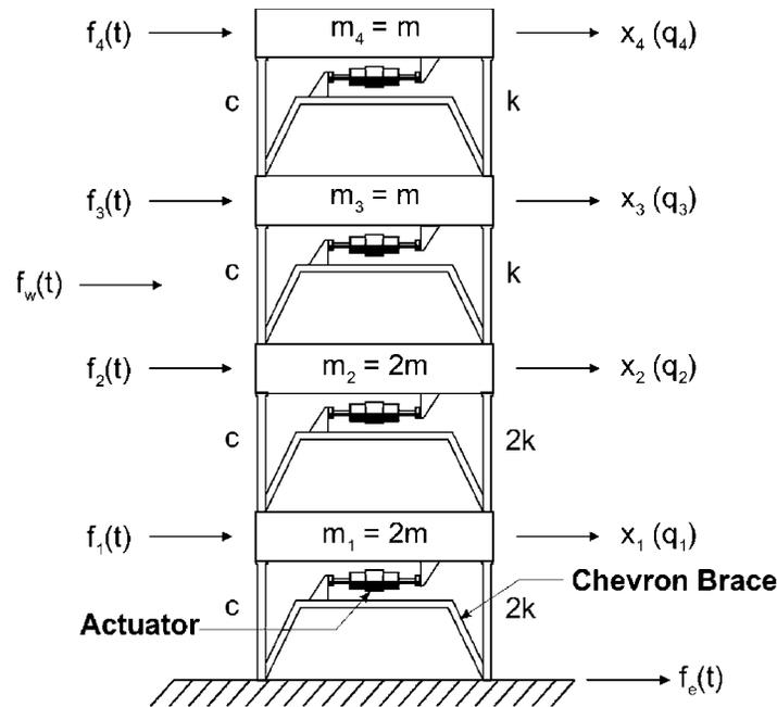
Figure 5.1. Building model for numerical example.
