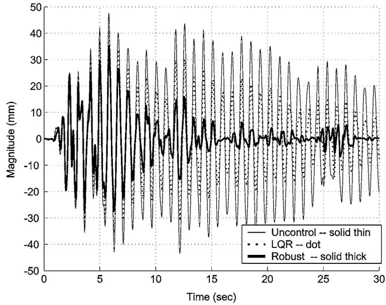
**Figure 7.3.** Perturbed model: Uncontrolled and controlled interstory drift of the 4-th floor.
