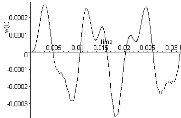
**Figure 5.2a.** Transverse displacement of free end of **delaminated** cantilever beam, excited by piezoelectric actuator. Beam length is  $L = 0.2m$ ,  $x$ -coordinates of the crack tips are  $\alpha = 0.1m$  and  $\beta = 0.15m$ ,  $z$ -coordinate of the crack tips is  $\gamma = 0.00165m$ . Linear analysis. **Both types of nonlinearity** are taken into account: due to non-penetration constraint and due to longitudinal force resultants.
