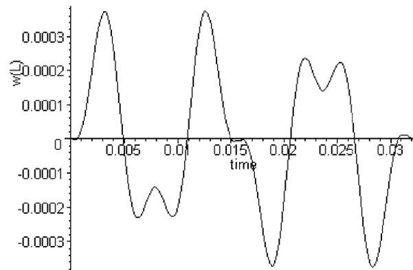
**Figure 5.3b.** Transverse displacement of free end of **undelaminated** cantilever beam, excited by piezoelectric actuator. Beam length is  $L = 0.2m$ ,  $x$ -coordinates of the crack tips are  $\alpha = 0.1m$  and  $\beta = 0.15m$ ,  $z$ -coordinate of the crack tips is  $\gamma = 0.001165m$ . **Nonlinear analysis.**
