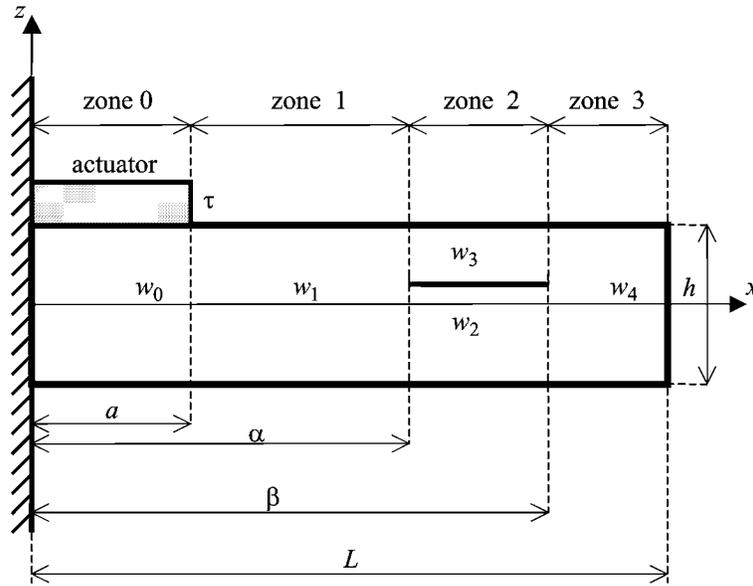
**Figure 4.1.** Cantilever beam with delamination and piezoelectric actuator.
