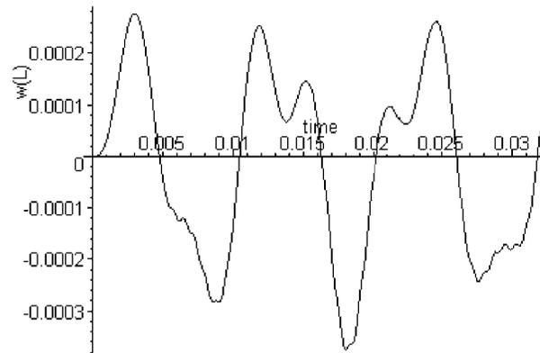
**Figure 5.1b.** Transverse displacement of free end of **delaminated** cantilever beam, excited by piezoelectric actuator. Beam length is  $L = 0.2m$ ,  $x$ -coordinates of the crack tips are  $\alpha = 0.1m$  and  $\beta = 0.15m$ ,  $z$ -coordinate of the crack tips is  $\gamma = 0.00165m$ . **Nonlinear analysis.**
