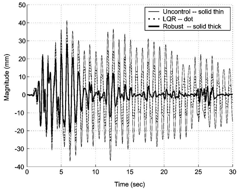
**Figure 7.1.** Nominal model: Uncontrolled and controlled interstory drift of the 4-th floor.
