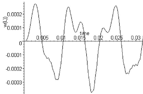
**Figure 5.2b.** Transverse displacement of free end of **delaminated** cantilever beam, excited by piezoelectric actuator. Beam length is  $L = 0.2m$ ,  $x$ -coordinates of the crack tips are  $\alpha = 0.1m$  and  $\beta = 0.15m$ ,  $z$ -coordinate of the crack tips is  $\gamma = 0.00165m$ . Nonlinear analysis. **Only one types of nonlinearity** is take into account: due to non-penetration constraint.
