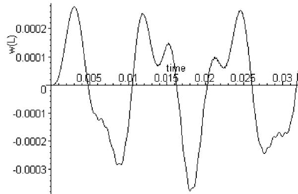
**Figure 5.3a.** Transverse displacement of free end of **delaminated** cantilever beam, excited by piezoelectric actuator. Beam length is  $L = 0.2m$ ,  $x$ -coordinates of the crack tips are  $\alpha = 0.1m$  and  $\beta = 0.15m$ ,  $z$ -coordinate of the crack tips is  $\gamma = 0.001165m$ . **Nonlinear analysis.**
