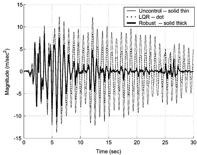
**Figure 7.2.** Nominal model: Uncontrolled and controlled absolute acceleration of the 4-th floor.
