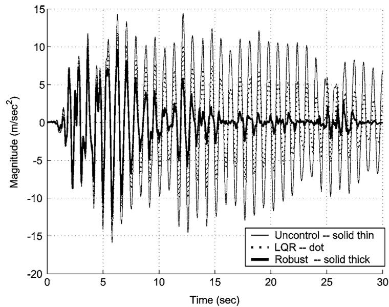
**Figure 7.4.** Perturbed model: Uncontrolled and controlled absolute acceleration of the 4-th floor.
