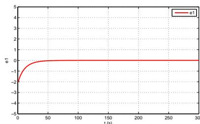
**Figure 4:** Time-response of the error  $e_1(t)$  under the controller (35) for *FSHP*.
