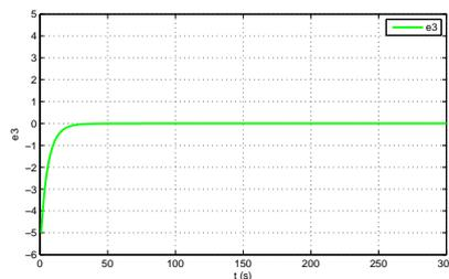
**Figure 6:** Time-response of the error  $e_3(t)$  under the controller (35) for *FSHP*.
