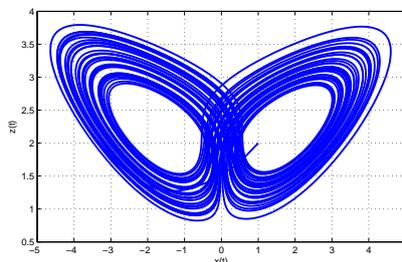
**Figure 1:** Simulation result for the fractional-order system (7) projected onto the  $x - z$  plane.
