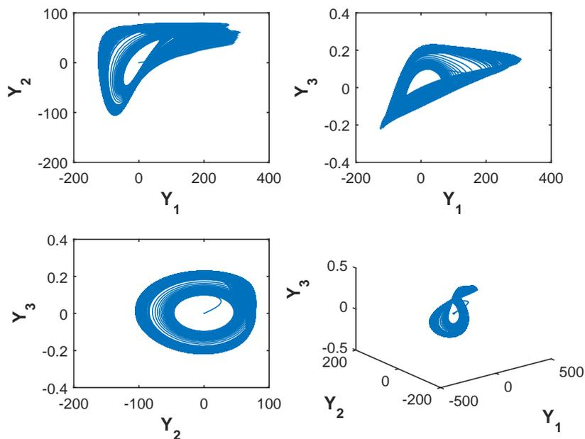
**Figure 2:** Phase space realization of Chua's circuit with the memristor of the form  $W_i = -a + 3by_4^2$ , where the values of  $a$  and  $b$  are taken as  $0.6667 \times 10^{-3}$  and 1.4828, respectively.
