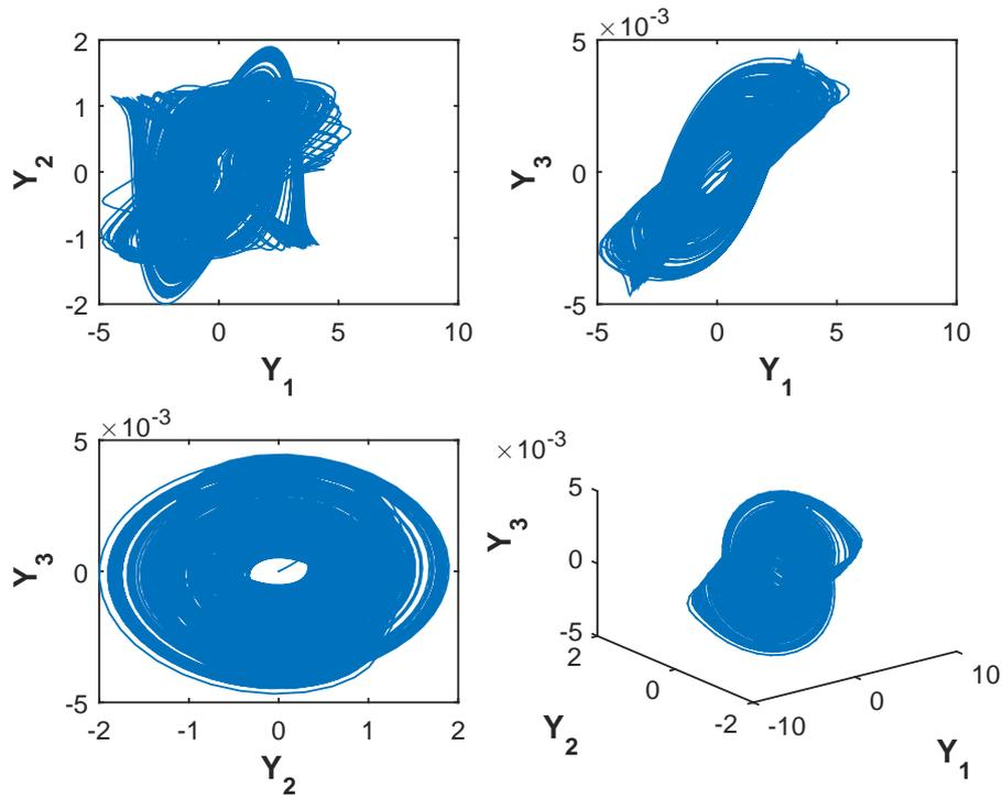
**Figure 1:** Phase space realization of Chua’s circuit with a memristor of the form  $W_i = -a+b|y_4|$ , where the values of  $a$  and  $b$  are taken as  $0.6667 \times 10^{-3}$  and  $1.4828$ , respectively.
