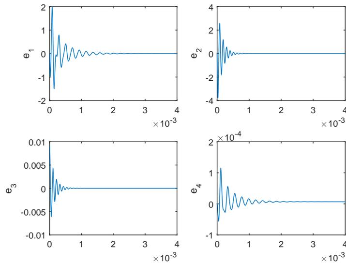
**Figure 4:** The synchronization error functions for two systems with the memristor of type I using control functions as described in Corollary 3.1.
