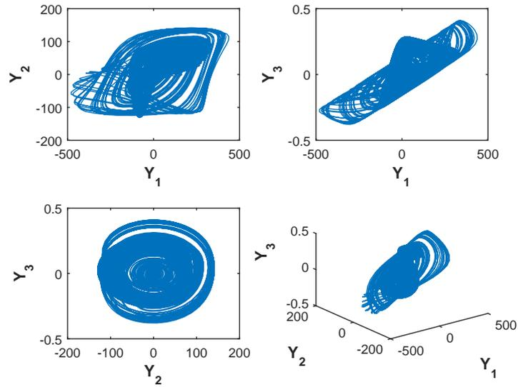
**Figure 3:** Phase space realization of Chua’s circuit with memristor of the form  $W_i = ay_4^4 - by_4^2 - c$ , where the values of  $a$   $b$  and  $c$  are taken as 1000, 1.087 and  $0.33e^{-3}$ , respectively.
