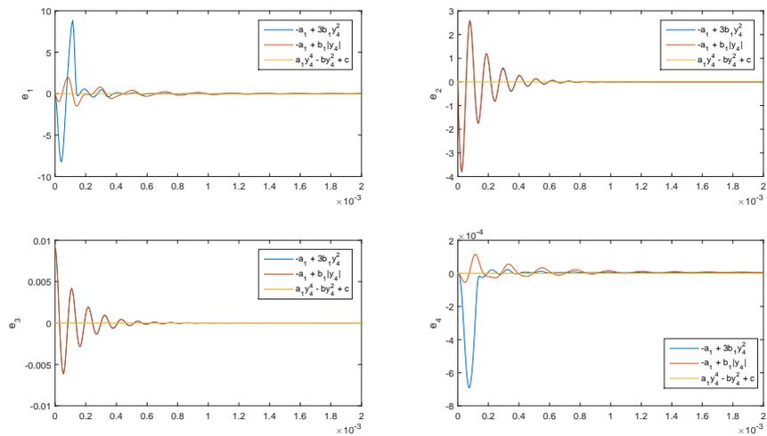
**Figure 7:** Error functions of different memristors when synchronized with the memristor  $W_{ii}$  (where  $i = 1, 2, 3$ ).
