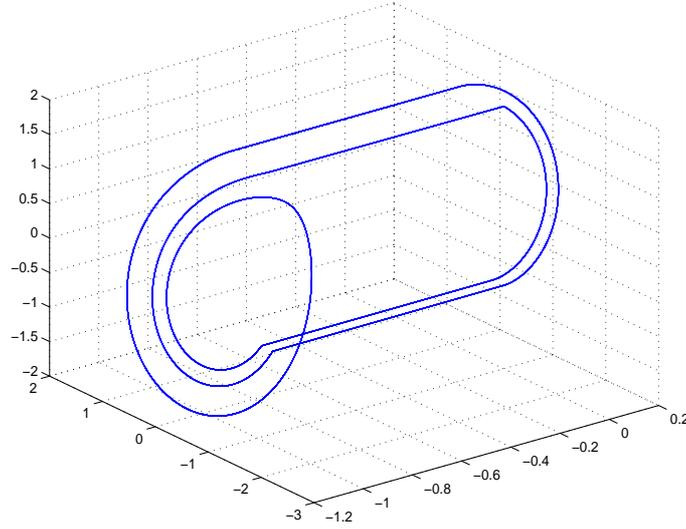
**Figure 2:** Symmetric sliding case: period doubling for  $\varepsilon = 0.2$
