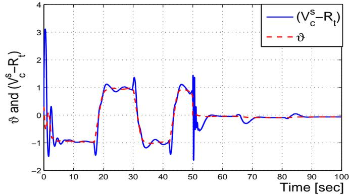
Figure 3: Identification of uncertainties ( $\vartheta$ ) by NN ( $V_c^s - R_t$ ).
