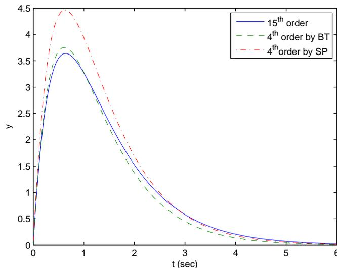
**Figure 5:** The output of the circuit bilinear system, BT: balanced truncation, SP: singular perturbation.
