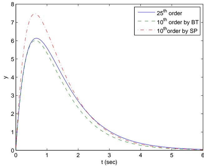
**Figure 3:** The output of the circuit bilinear system, BT: balanced truncation, SP: singular perturbation.
