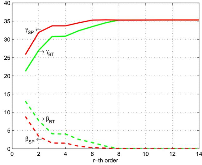
Figure 2: The  $H_2$ -norm  $\beta$  and least upper bound  $\gamma$  of the difference bilinear system.
