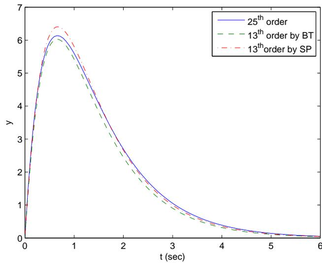
**Figure 4:** The output of the circuit bilinear system, BT: balanced truncation, SP: singular perturbation.
