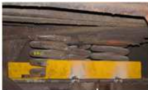
Figure 4: Secondary spring system.
