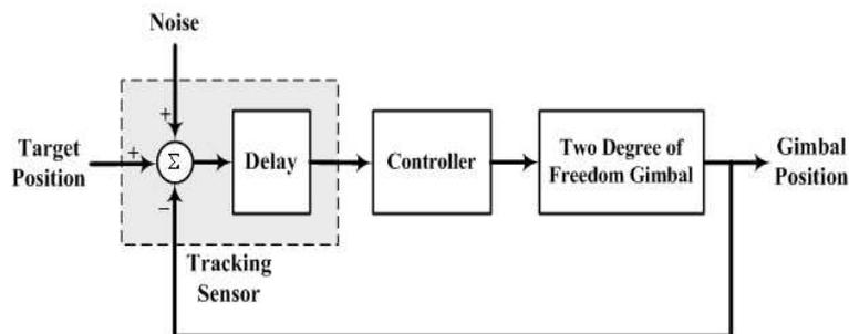
**Figure 1:** A simple diagram of tracking loop.
