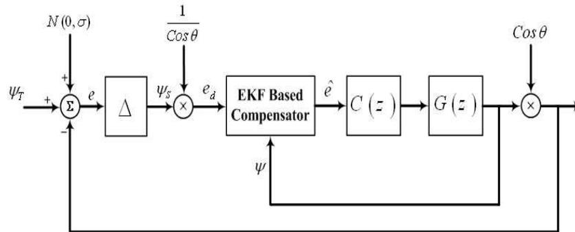
Figure 4: Mathematical model of tracking loop structure.
