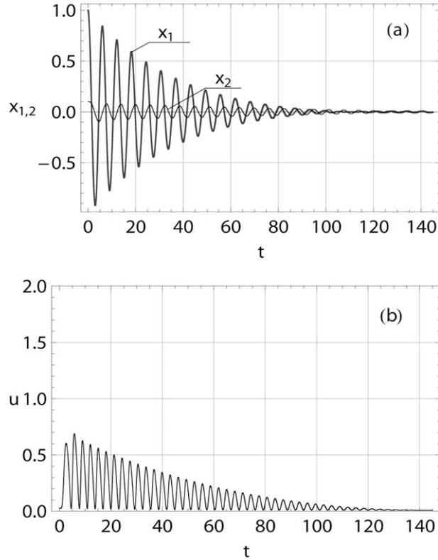
**Figure 4:** Beat suppression under the reduced time increment  $h = 0.001$  but increased weight parameter  $\lambda = 10.0$ : (a) the system response, (b) control input - the damping ratio of second oscillator.
