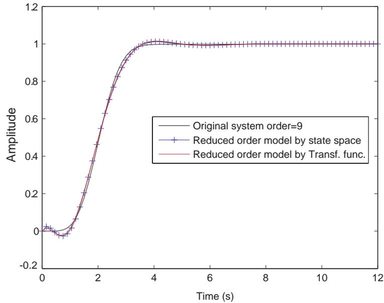
**Figure 1:** Step responses of the original system order  $n = 9$  and reduced order models  $r = 3$  obtained by the proposed techniques : starting from a state space realization and from a transfer function.
