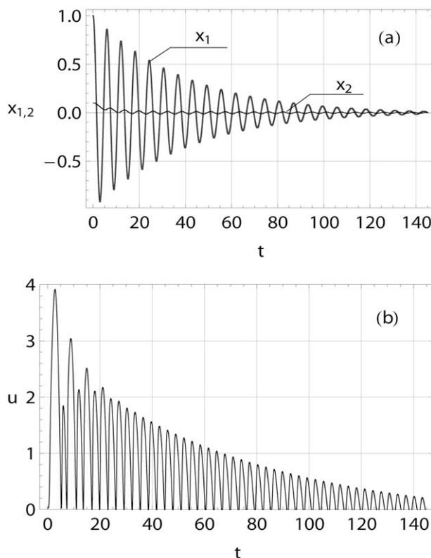
**Figure 5:** Beat suppression under the reduced time increment  $h = 0.001$  and vanishing weight parameter  $\lambda = 0.1$ : (a) the system response, (b) control input - the damping ratio of second oscillator.
