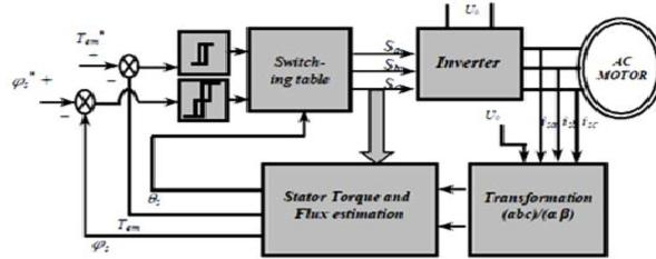
**Figure 1:** Schematic diagram of CDTC strategy.
