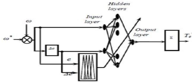
Figure 6: Basic structure of neural fuzzy speed controller.
