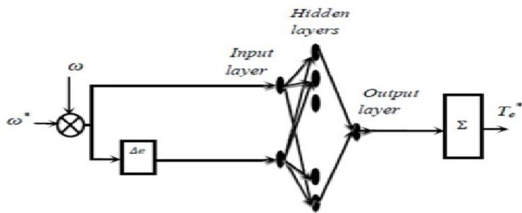
Figure 7: Basic structure of neural speed controller.
