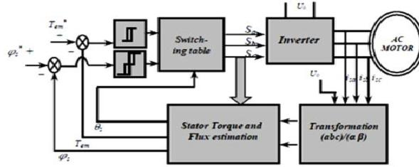
**Figure 1:** Schematic diagram of CDTC strategy.
